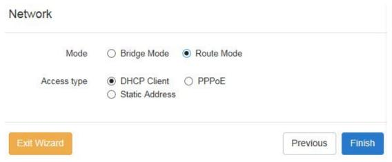
a. DHCP Client: It automatically gets the IP address assigned by the superior gateway.
