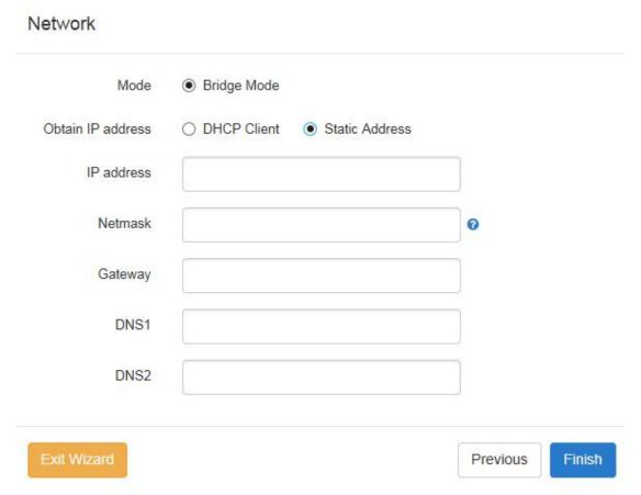
b. Static Address: Under the mode, you need to set the information manually, including IPv4 address, netmask, Gateway, DNS.
