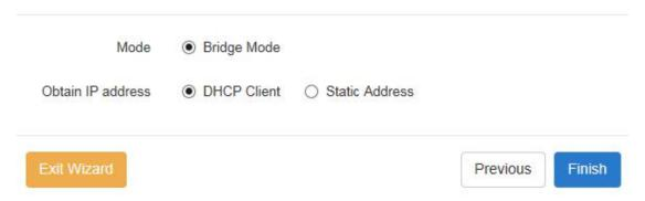
a. DHCP Client: It automatically gets the IP address assigned by the superior router.
