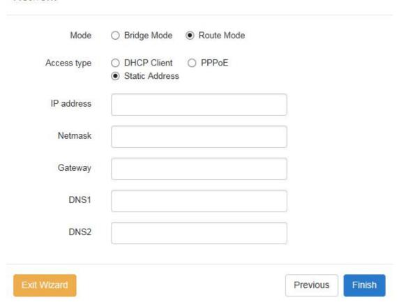
c. Static Address: Under the mode, you need to set the information manually, including IPv4 address, netmask, Gateway, DNS.
